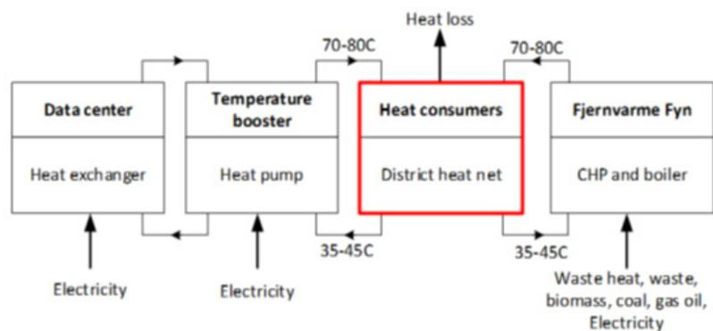
Figure 1: The structure of the heat pump plant and interaction with other production plants.
