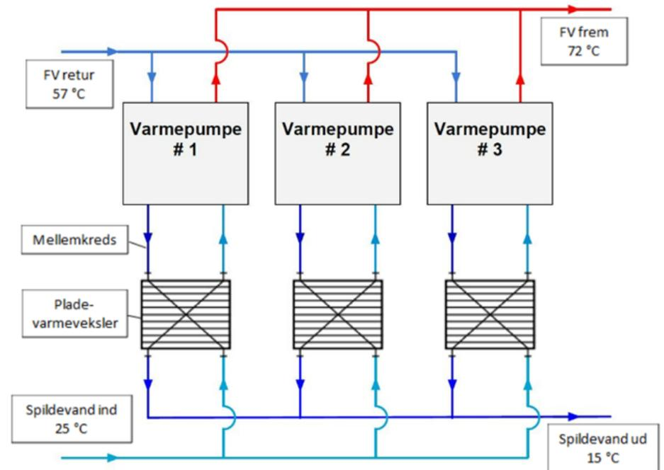
Figure 6: Plant construction in Kalundborg. The three parallel heat pumps are seen at the top, where the district heating water enters from the left and is delivered to the inlet on the right. Below the heat pumps are the plate heat exchangers, which separate the waste water from the intermediate circuit.
