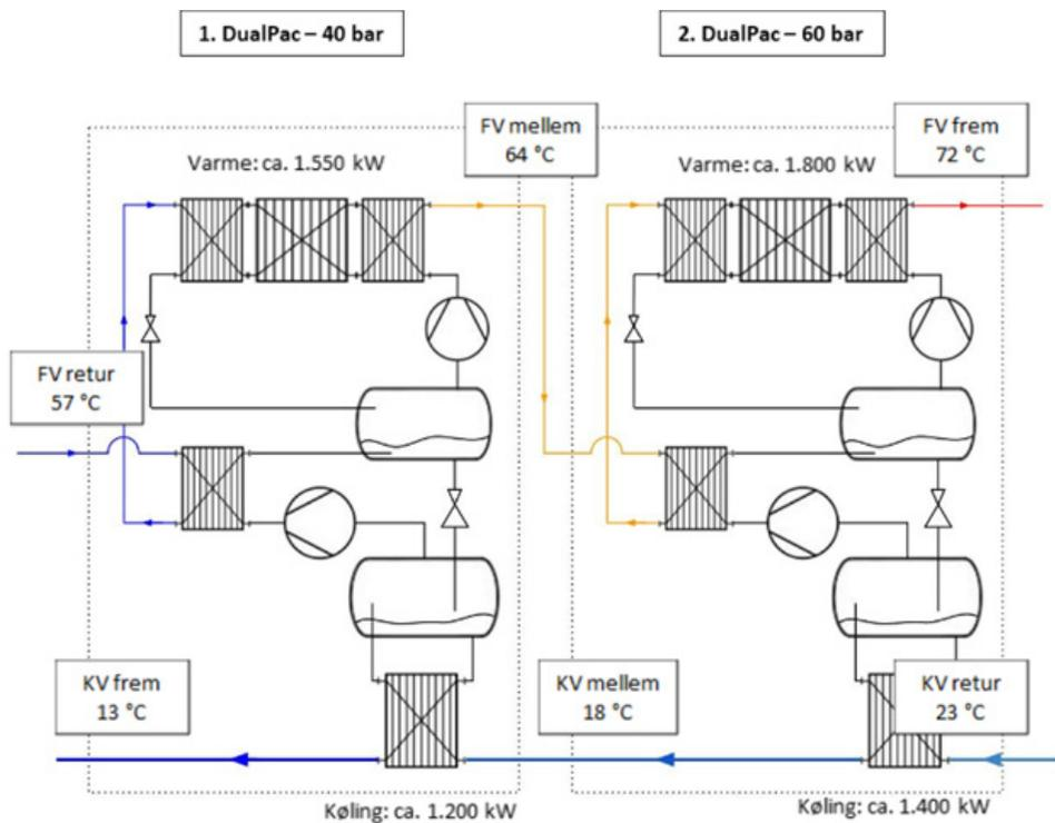
**Figure 7:** Principle sketch of the heat pump system in Kalundborg. The figure shows one out of three identical sets.
